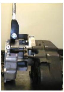
"T" handle linkage installed
