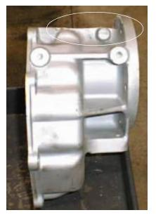
Modified to fit the transfer case shifter linkage
