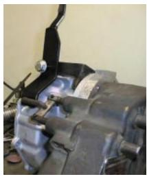
"T" handle linkage installed
